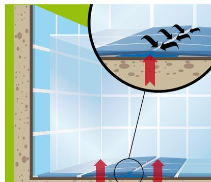
Tiling onto under floor heated systems; the tiles usually have a lower coefficient of thermal expansion. For a given temperature rise tiles will expand less than the substrate and stresses will be formed at the interface between the tile and the adhesive. At weak bonded parts, the tiles may delaminate or blow away from their base. Same rule applies for the substrates on heat transmitting systems and insulation applications.
