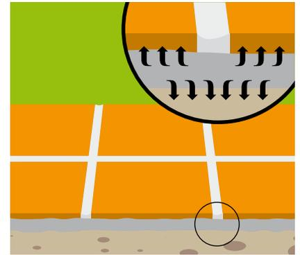
When tiling is done with a standard performance adhesive onto an impervious substrate, the adherence is much weaker resulting in tiles de-bonding from the substrate.
