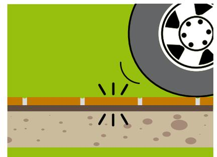
Any area of the tile that has no contact on the substrate and has voids is vulnerable when subjected to a localized load. These fragile points will let cracks and crashes of the covering.
