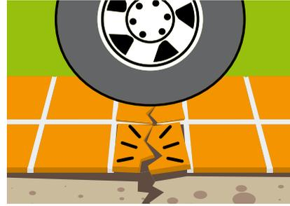
■ Any area of the tile that has no contact on the substrate and has voids is vulnerable when subjected to a localized load. These fragile points will let cracks and crashes of the covering.
