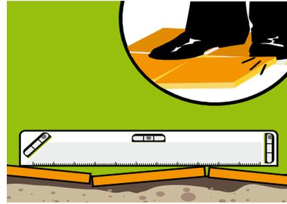
The substrate should be smoothed and stabilized with either surface repairing and smoothing plasters or leveling compounds.
