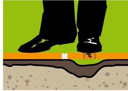
■ If the substrate is not leveled, this will cause edges on the covering. The edges will affect aesthetics of the covering and block motion.
